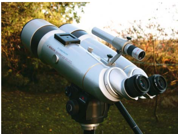
Figure 7.2. 3×12 finder scope with 55-mm eye relief.
