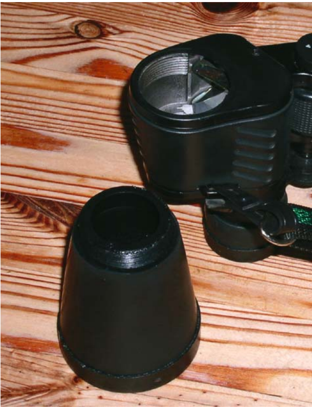
Figure 5.3. Objective barrel unscrewed. The prisms are visible under the cover plate.
