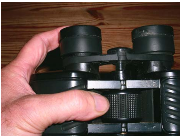
Figure 2.27. The bridge rocks on this center-focus Porro prism binocular.
