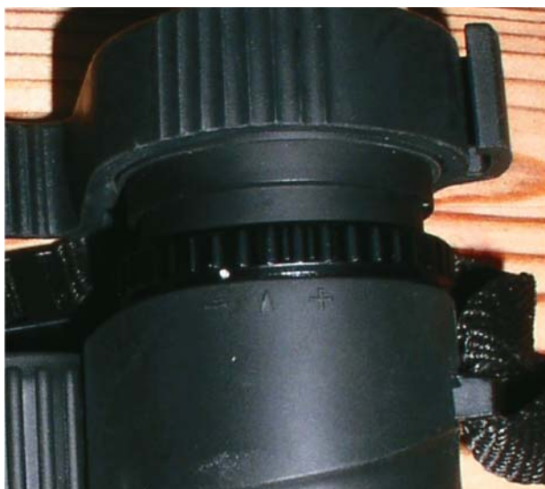
Figure 2.26. Right eyepiece dioptric adjustment. a: Porro prism. b: Roof prism.
