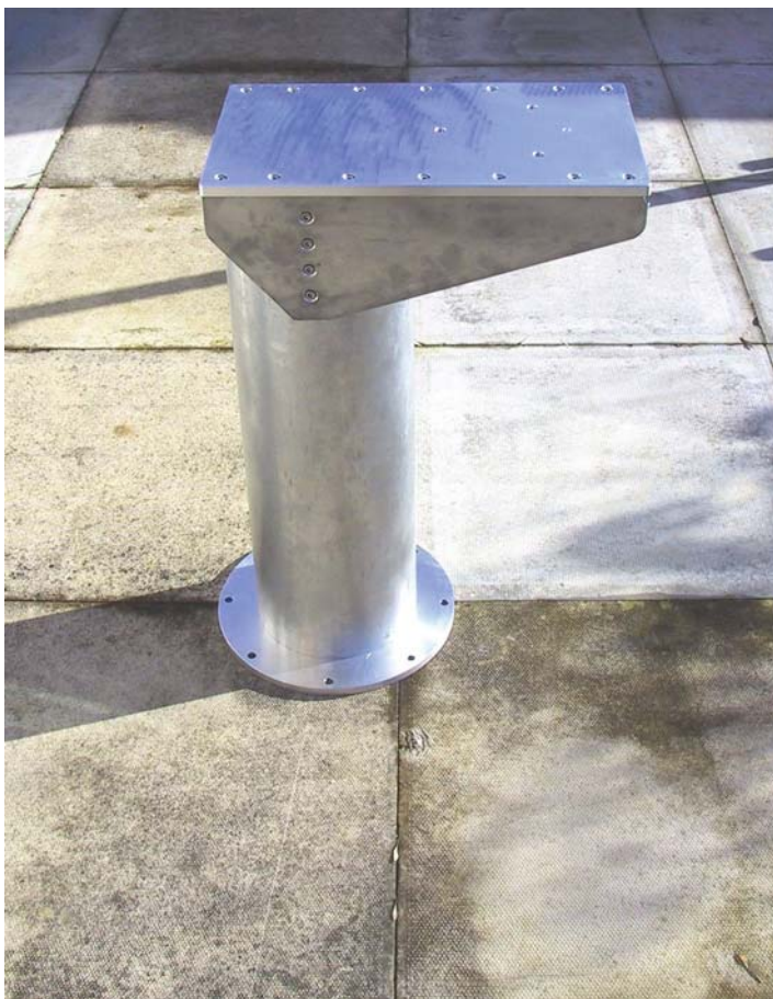
Figure 1.3. The custom-made all-aluminium Equatorial mode pillar.
