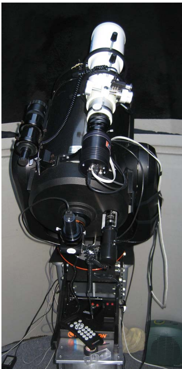
Figure 1.6. The Sky 90 f#4.5 refractor system mounted piggyback on the Nexstar11 GPS.
