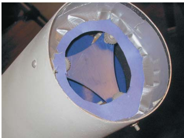
Plate 17. Simple mirror-end baffle for Newtonian.
