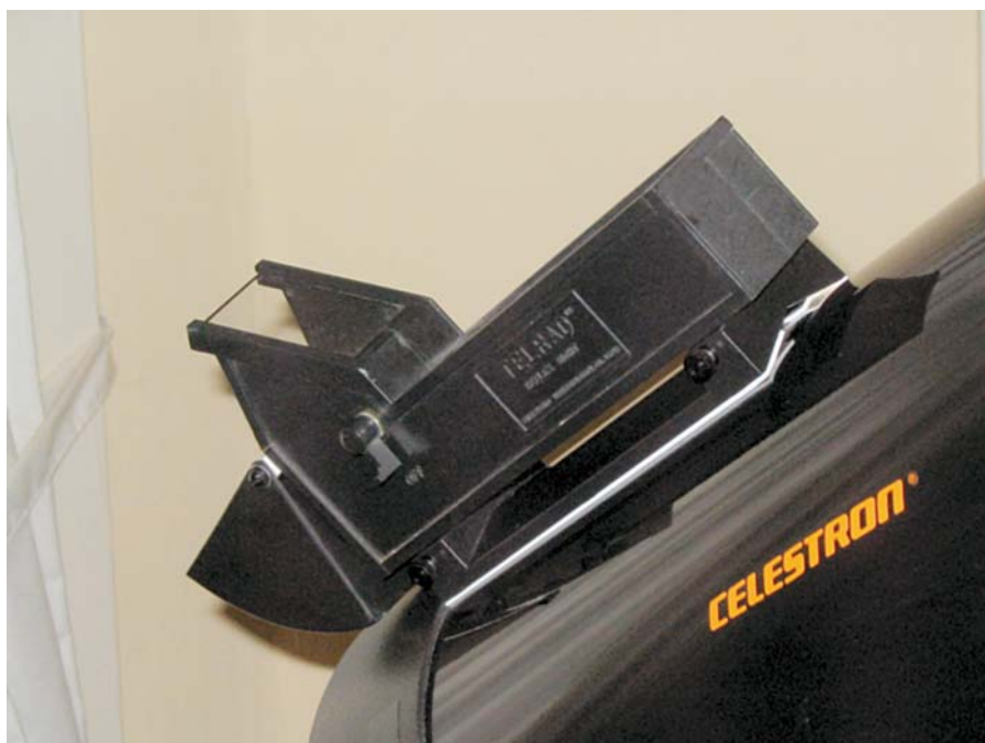
Plate 10. Steve Kufeld's ingenious TELRAD aiming device.
