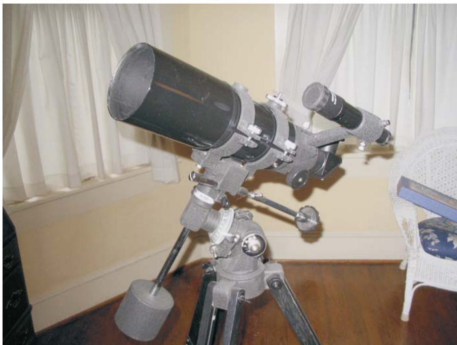
Plate 2. Celestron's 80 mm f/5 refractor.
