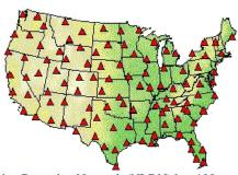
National Lightning Detection Network (NLDN) has 108 sensors throughout United States. Graphic courtesy LightningStorm.com and Global Atmospherics, Inc.
