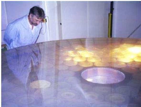
SOFIA's Zerodur f/1.28, 2.7 meter diameter Primary Mirror. Photograph courtesy of NASA.
