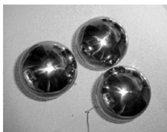
Photograph of experimental assembly with stainless-steel spheres. Two spheres are free to rotate about an axis perpendicular to the plane connecting the centers of the three spheres. The third sphere
