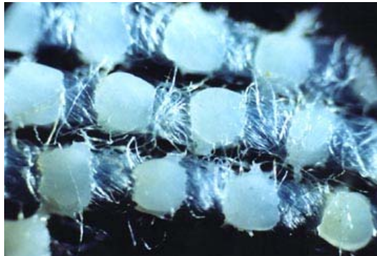
10 Second Test Top Surface: Sample from Corguinho, Brazil bed sheet which Phyllis Budinger subjected to iron test for 10 seconds. The melted polyester is flat and segmented, compared to the fluid weave of the vitreous threads in Sample 1 of the originally affected bed sheet above. Photomicrograph © 2003 by W. C. Levengood.
