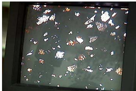
All the white objects with the tattered edges are quartz crystals which have been eroded by emersion in hot, liquid iron (approximately 2,000 degrees F.). Video image © 2003 by Linda Moulton Howe and Bob Terrio.
