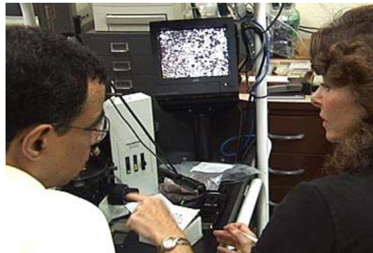
All the white grains on the petrographic microscope monitor are quartz crystals embedded in iron. Video image © 2003 by Linda Moulton Howe and Bob Terrio.
