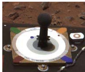
Martian calibration target in which the green, orange, blue and red tabs match well to the same tab colors on Earth. This means that the red of the soil and rock colors are close to true color.
