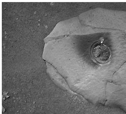
Circular area cleared of red dust was ground by Spirit's robotic grinding tool .
