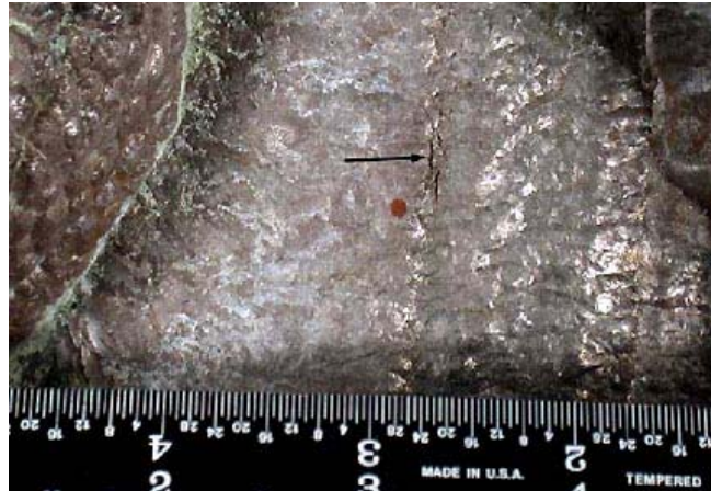
Arrow points to crack in 6-inch steel cladding at Nozzle # 3, Davis-Besse Nuclear Power Plant, 2002. Photograph by Nuclear Regulatory Commission.
