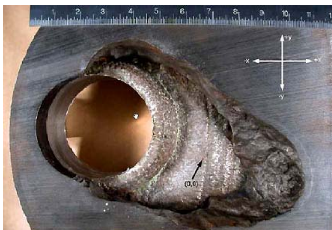
Leaking boric acid ate a 6-inch wide hole around the steel cladding of Nozzle #3 in the reactor head at the Davis Besse nuclear power plant near Toledo, Ohio. Discovered in 6-inch steel casing and photographed in March 2002. Plant shut down to avoid potential core melt down. Photograph from Nuclear Regulatory Commission .
