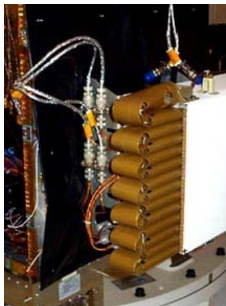
MARSIS main antenna during Mars Express payload tests. NASA describes, "One of the two main radar booms is shown here, a 20-meter long hollow cylinder folded up in a box like an accordion. When the box is opened, the elastic energy of the compressed glass-fibre booms will let them unfold like a jack-in-the-box." Image credit: University der Bundeswehr, Germany.
