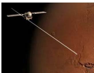
Mars Express spacecraft in orbit around Mars with graphic of the Mars Advanced Radar for Subsurface and Ionosphere Sounding (MARSIS) antennas unfurled. The third and most recent was successfully deployed on June 17. ESA radar will "see" into top 3 miles (5 kilometers) of
