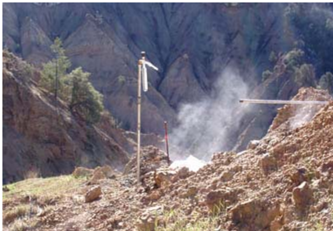
Gas sample tube on the wellhead. Maximum temperature measured was at 11.5 feet underground at 584 degrees F. Photograph courtesy Robert H. Mariner, USGS.
