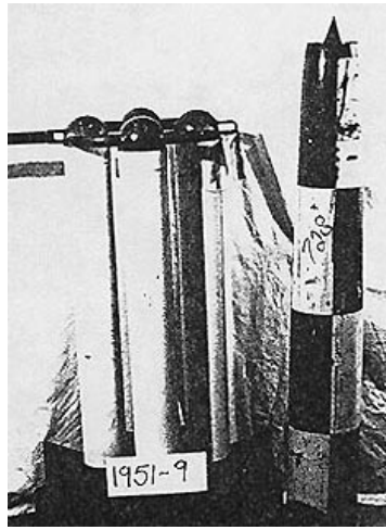
Original full-scale replica of America's first surface-to-air missile, the Supersonic Test Vehicle (STV), called Bumblebee, or the "Flying Stovepipe." Demonstration flight was on October 16, 1945, Island Beach, New Jersey, and reached 1400 mph. Produced by Johns Hopkins University Applied Physics Laboratory, Baltimore, Maryland.
