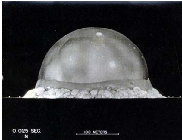
Early stage of Fat Boy "gadget" atomic bomb test on July 16, 1945, at Trinity Site, WSPG, which detonated at 05:29:45 local Mountain War Time with energy equivalent to 19 kilotons of TNT. The Seattle Times : "The heat was so intense that it vaporized the tower holding the bomb and melted the sand underneath into a green glass dubbed Trinitite. A mile away, exposed surfaces were heated to 750 degrees. At 10 miles, the heat still felt like the open mouth of a fireplace, witnesses reported. Despite bulldozing away the fused sand, the radiation levels today, half a century later, are still ten times that of the background radiation levels found in nature from radioactive rocks and cosmic rays."
