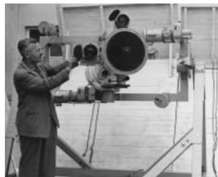
Astronomer Clyde Tombaugh designed, produced and operated optical telescopes at WSPG to resolve V-2 rockets in flight at 160 kilometers (99 miles). Photograph from NMSU Library.
