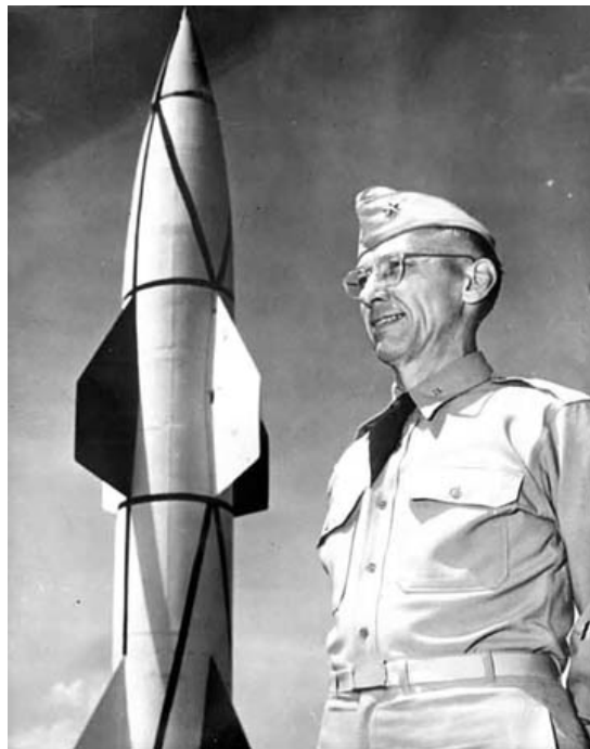
Major Holger Toftoy, Chief of U. S. Army-Ordnance, Enemy Equipment Intelligence Section (EEIS), in front of a German Wasserfall rocket modified by the American Project PAPERCLIP at WSPG and called an Hermes A-1 surface-to-air missile.
