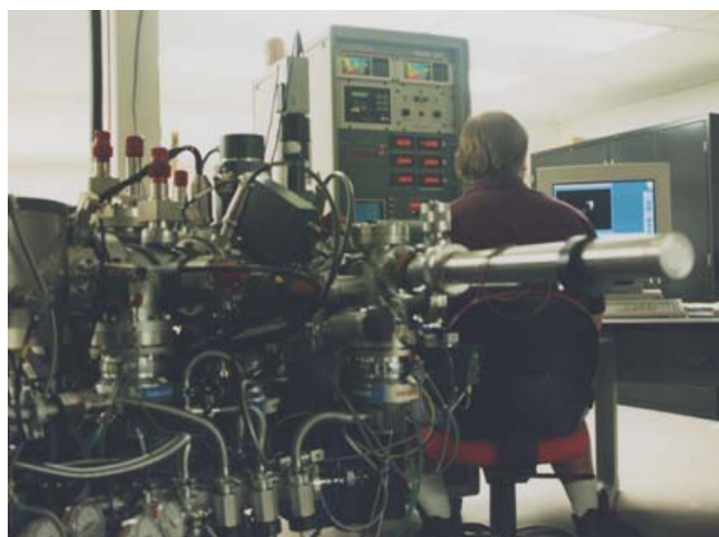
Ion microprobe and Eric Hauri, Ph.D., at Carnegie Institution of Washington, D. C., July 20, 1996, during magnesium isotope ratio analysis of bismuth and magnesium/zinc layered metal. Photograph © 1996 by Linda Moulton Howe.
