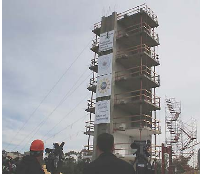
January 14, 2006 "shake table" test of 7-story building built specifically to test its strength in a seismic shaking equivalent to the January 17, 1994, Northridge earthquake. It was a 6.7 magnitude quake that killed 60 people, injured 7,000, left 20,000 homeless, and damaged more than 40,000 buildings in Los Angeles, Ventura, Orange and San Bernardino Counties. Image courtesy UCSD.
