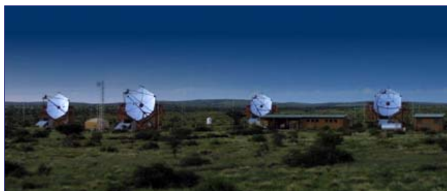
High Energy Stereoscopic System (H.E.S.S.) system of Imaging Atmospheric Cherenkov Telescopes for investigation of cosmic gamma rays in the 100 GeV energy range. First operation began in Summer 2002 in Gamsberg, Namibia. Image courtesy H.E.S.S.
