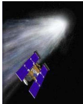
Stardust spacecraft flew through Comet Wild 2 dust in 2000, 2002 and 2004, collecting particles in aerogel. Image and graphic courtesy NASA.
