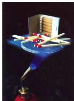
Matches on top of aerogel disc above a gas torch flame illustrate the excellent insulating properties of aerogel. The aerogel used
