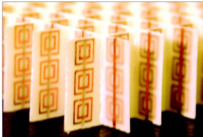
Metal lattice of "perfect lens." Image courtesy University of California, San Diego.
