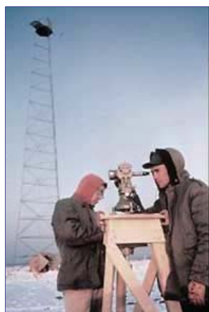
Left: Circa 1950, U.S. National Geodetic Survey technicians observing with a 0.2 arcsecond resolution Wild T-3 theodolite mounted on an observing stand. Photo was taken during an Arctic field party. Credit: NOAA. Right: An optical theodolite, manufactured in the Soviet Union in 1958 and used for topographic surveying. ]
