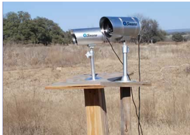
Infrared camera on left is Swann 16mm 1/3 IR CS 1:1.6. Camera on right is Swann 16mm CCTV F1.2. The two camera lenses are 28 inches apart. The cameras are about five feet above ground and mounted on wooden posts that set on a base of rocks. Photograph © 2008 by Linda Moulton Howe.
