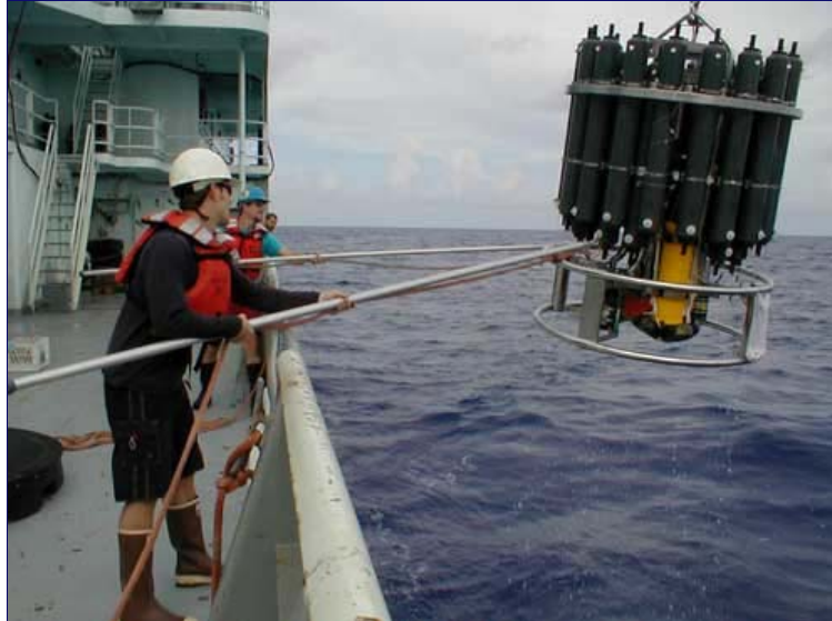
NOAA research team recovered the water sampling package called a rosette. Each of the gray cylinders can be closed at whatever depth the scientists choose. Each bottle traps 11 liters of water that can then be sub-sampled by the various analysts on the ship for a variety of measurements. Image courtesy NOAA.
