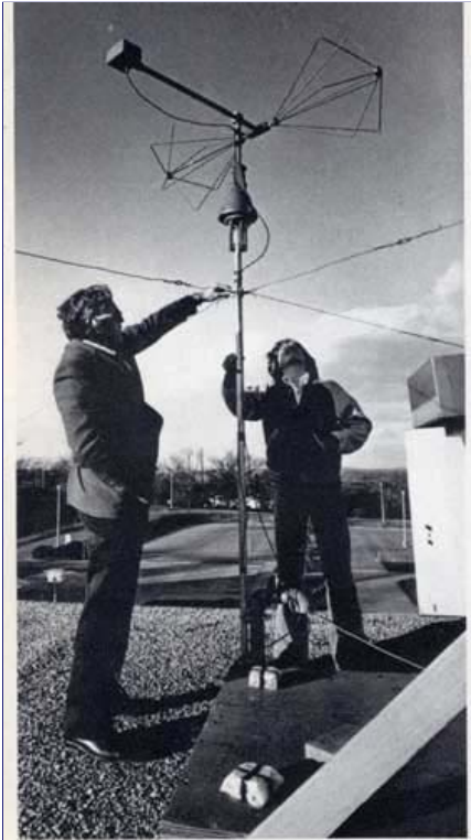
Plate 35. I tighten a guy wire while Mark watches. The biconical antenna connects to a spectrum analyzer. Other detectors on the roof are a Geiger counter tube, radio antenna, and magnetometer pickup coil. (By permission of St. Louis Post-Dispatch; Gene Pospeshil)
