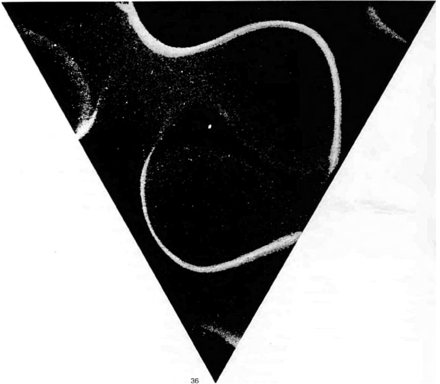
36 A sonorous figure produced by piezoelectric excitation. The triangle measures 24 cm along each edge. Steel plate. Frequency 875 cps.
