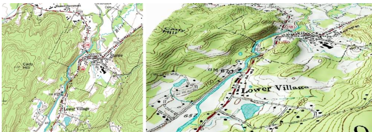
o / Left: A topographical map of Stowe, Vermont. From one constant-height line to the next is a height difference of 200 feet. Lines far apart, as in the lower village, indicate relatively flat terrain, while lines close together, like the ones to the west of the main town, represent a steep slope. Streams flow downhill, perpendicular to the constant-height lines. Right: The same map has been redrawn in perspective, with shading to suggest relief.
