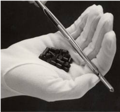
e / These pellets of uranium fuel will be inserted into the metal fuel rod and used in a nuclear reactor. The pellets emit alpha and beta radiation, which the gloves are thick enough to stop.
