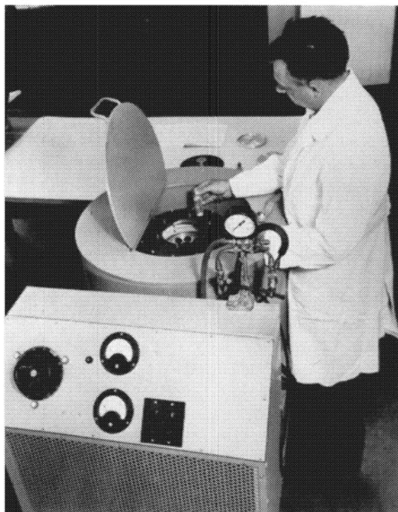
Figure 28 Crellen Laboratory's high-speed centrifuge (20,000 rpm) for molecular studies of proteins. Courtesy of the Rockefeller Archive Center.
