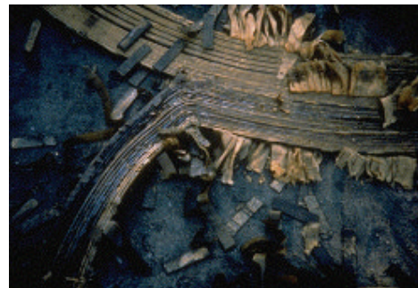
Figure 2-3. GIC Damage to Transformer During 1989 Geomagnetic Storm
