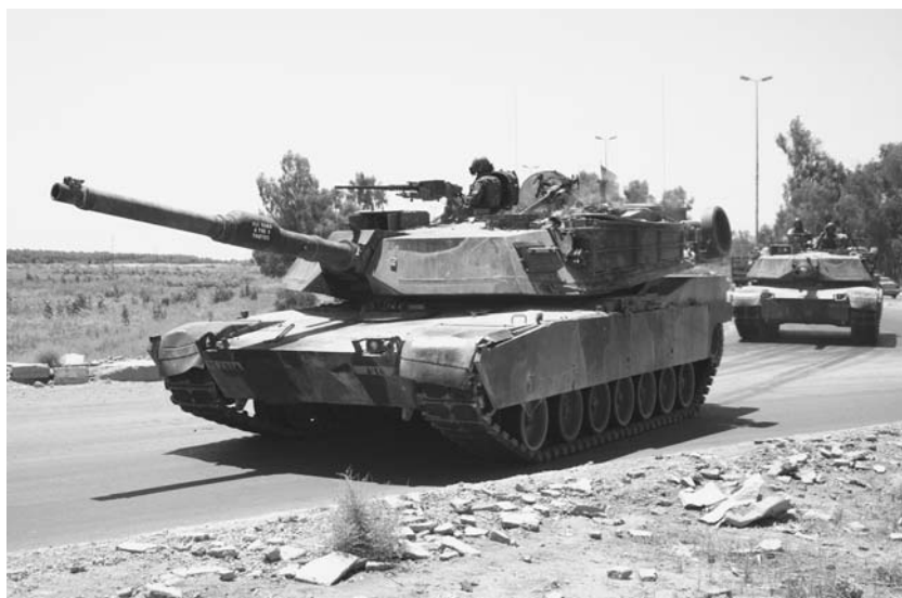
Armor made from layers of metal and other strong materials protects tanks such as the M1 Abrams. ( United States Army/Staff Sgt. Klaus Baesu )
