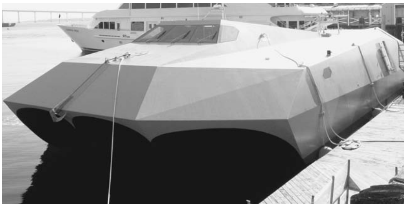
The hull of this experiment vessel is made from carbon composites, strong enough to withstand the pounding of waves during high-speed maneuvering. (Department of Defense/Samantha L. Quigley)
