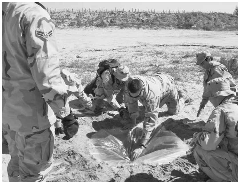
Soldiers deployed in the desert may need to supplement their water ration with a solar still. Sunlight passes through a transparent plastic cover and warms the ground, evaporating moisture that rises and condenses on the plastic. ( United States Air Force/Captain Karalyne Lowery )
