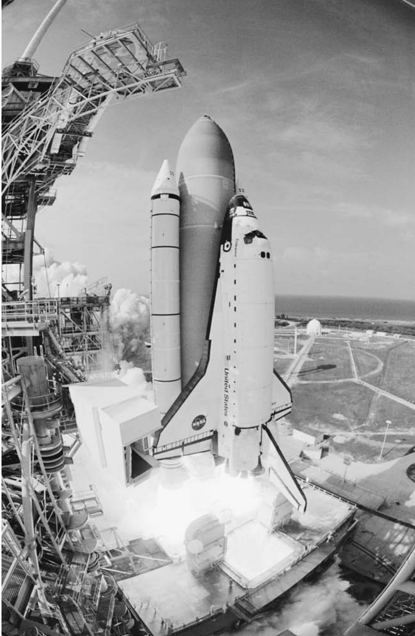
The space shuttle Endeavour lifts off on June 5, 2002. One of the two solid rocket boosters can be seen attached to the side of the external fuel tank, which is the large cylindrical object located underneath the shuttle. (NASA)
