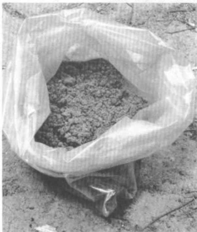
The powder is poured into a plastic bag for sun drying.
