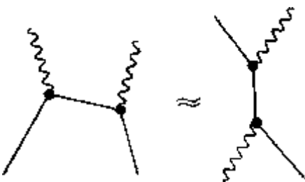
Fig. 25.10 Crossing symmetry. Processes which differ only with respect to the time-orderings in various places, but without the topology of the diagram being affected, are basically mathematically equivalent (through analytic continuation, §7.4). This is illustrated by such an equivalence between the particle–antiparticle pair annihilation into two photons, as illustrated on the left, and the Compton scattering process on the right (drawn without zigzags).
