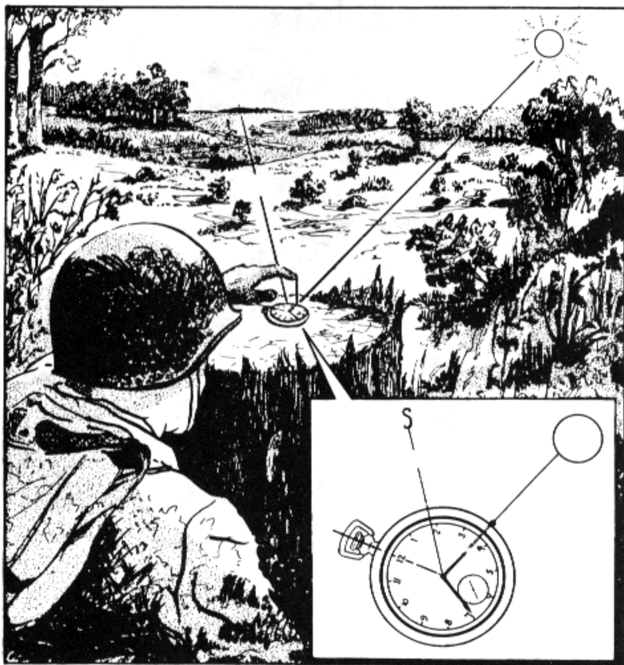
Figure 9. Sun and watch method of determining direction.
