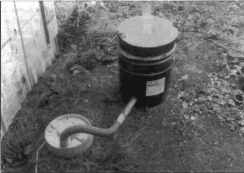
Figure 12-9. David Gingery's charcoal-fueled mini blast furnace. Illustration courtesy of The Charcoal Foundry by David J. Gingery (Gingery, 1983).
