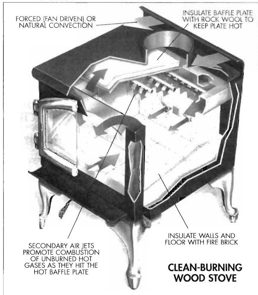
Figure 11-15. Clean-burning wood stove features. Illustration courtesy of Aladdin Hearth Products, manufacturers of Quadra-Fire wood stoves.
